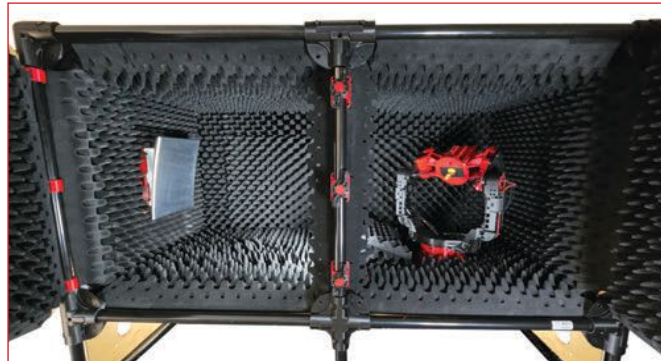
▲ Fig. 2 MilliBox MBX32CTR CATR.
