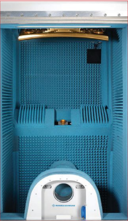
▲ Fig. 3 Rohde & Schwarz ATS1800C CATR. sional antenna tests, one of the most common strategies is to use someone else's antenna range. At first glance, this can seem like an inconvenient and expensive option
