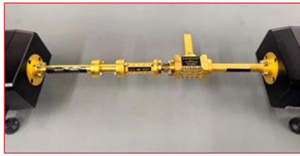
▲ Fig. 8 An OMT is an effective polarization filter for measuring the axial ratio.
