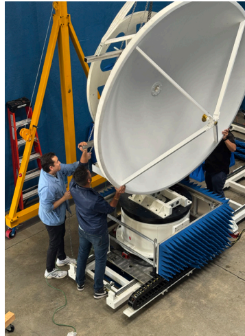
96" Cassegrain Antenna Being Loaded onto Near-Field Range
