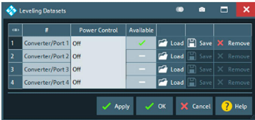
Fig. 4.4 – Level control should be disabled for all converters and ports.
