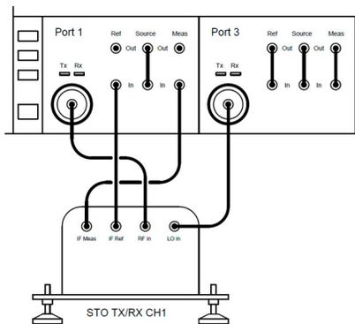
Fig. 3.2 – A single TX/RX frequency extender obtains an LO signal from Port 3 of the ZNA.
