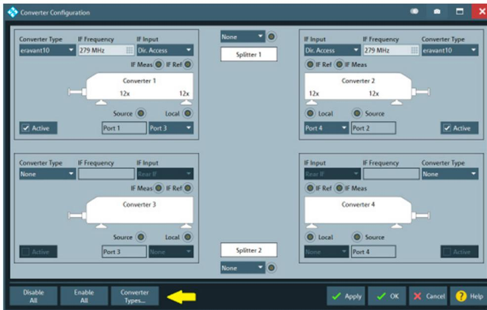
Fig. 4.1 – Select “Converter Types...” to edit an existing converter type or create a new one.
