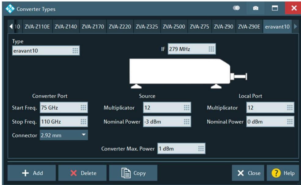
Fig. 4.2 – The “Converter Types” dialog captures the operating parameters of frequency converters.
