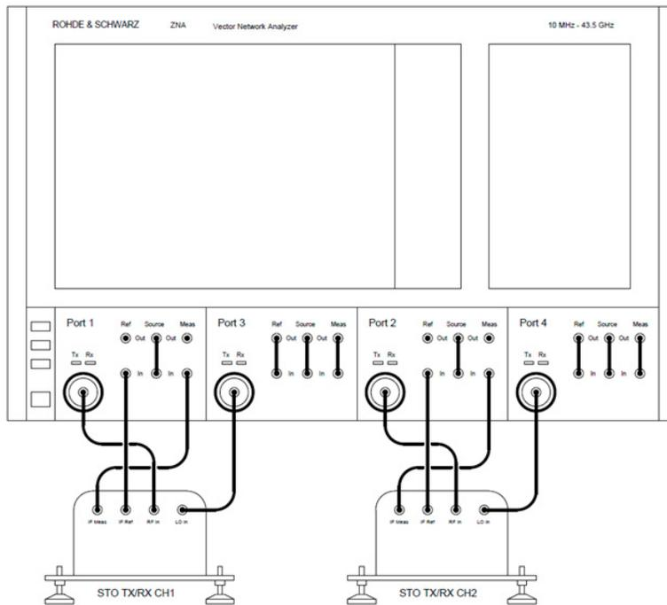
Fig. 3.1 – Each TX/RX frequency extender requires instrumentation-grade coaxial cables to carry the RF and LO signals to the extender, as well as the IF signals fed back to the VNA.
