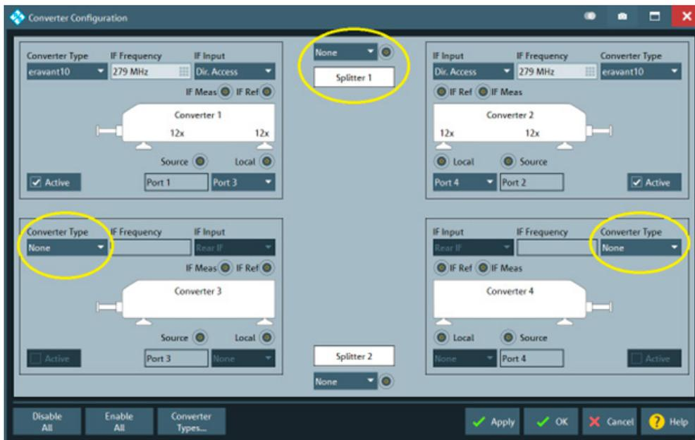
Fig. 4.3 – When two STO frequency extenders are connected to the front panel of a four-port ZNA, Converter 3 and Converter 4 are disabled by selecting “None” as the Converter Type. The “Splitter 1” data field should indicate “None”.
