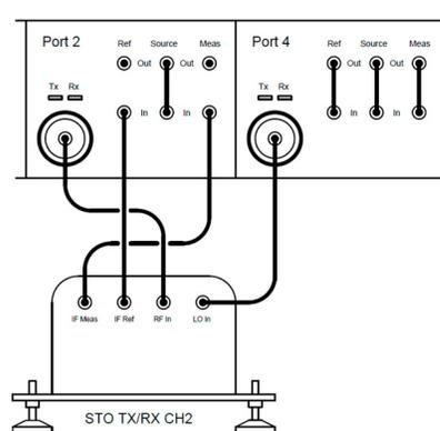
Fig. 3.3 – A second TX/RX extender obtains an LO signal from Port 4 of the ZNA. It is also possible to split the LO signal from Port 3 and apply it to both frequency extenders.
