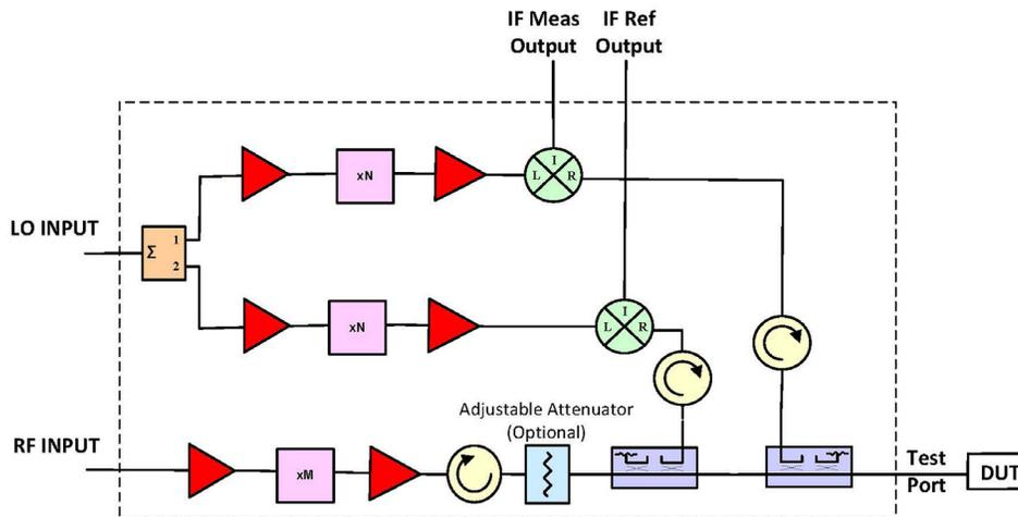
Fig. 1.1 – A single TX/RX frequency extender uses frequency multipliers to generate mm-wave test signals from lower frequency RF and LO signals provided by the VNA. Directional couplers sample the Reference and Measured signals. A pair of mixers down-convert the sampled signals to the IF of the VNA.
