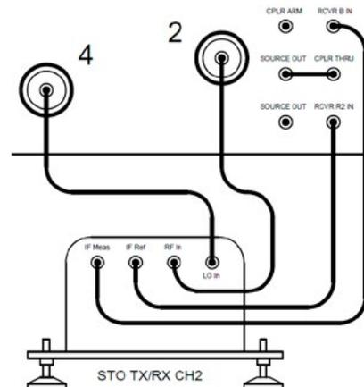
Fig. 3.3 – A second TX/RX extender obtains its LO signal from Port 4 of the PNA.
