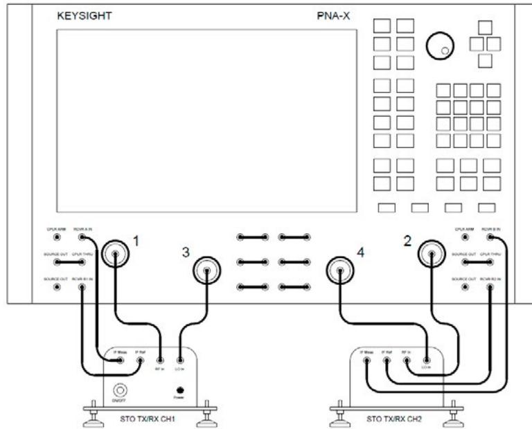
Fig. 3.1 – Each TX/RX frequency extender requires four instrumentation-grade coaxial cables to carry RF and LO signals to the extender and two IF signals back to the VNA. Ports 3 and 4 supply the LO signals.
