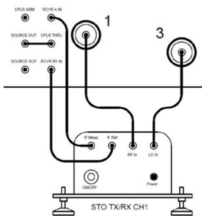
Fig. 3.2 – A single TX/RX frequency extender obtains its LO signal from Port 3 of the PNA.
