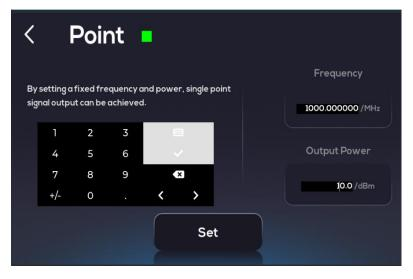
In the point frequency setting interface, you can enter the required frequency and power values, then press the Set button to apply the settings.
