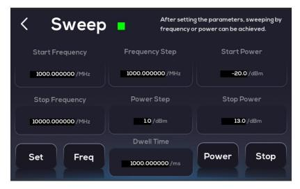
In the Sweep settings interface, you can enter the frequency and power of the start and stop points for the scan, as well as the step and dwell time values, and then press the Set button to apply the settings. You can choose between two scanning methods: frequency or power.
