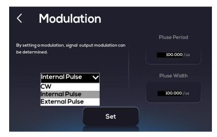
In the Modulation settings interface, you can set the modulation method. There are three modulation methods to choose from: continuous modulation, internal pulse, and external pulse modulation.
