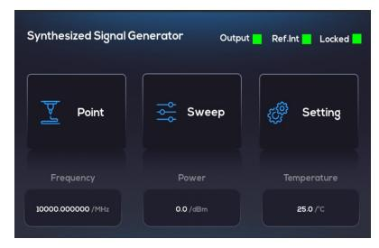
In the system's main interface, the current frequency, power, and temperature of the device will be displayed, along with the status of the output, reference source, and lock.
