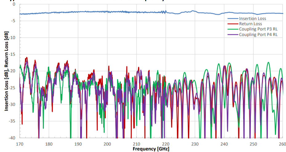
Typical Insertion Loss and Return Loss vs Frequency
