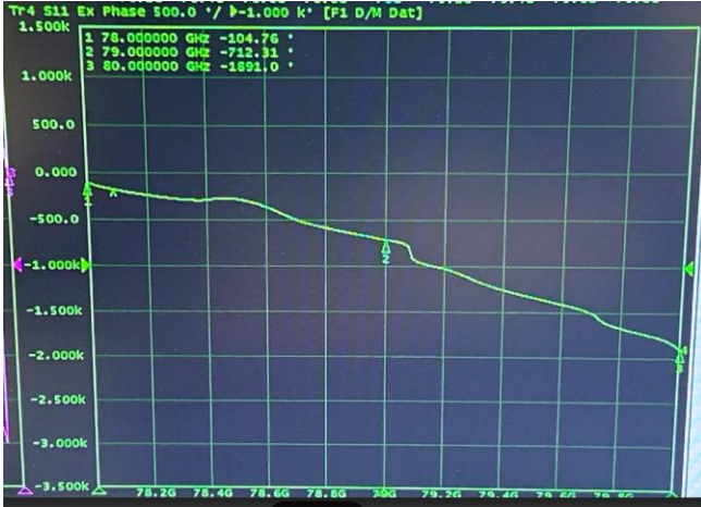
Fig. 4. Measured Phase Delay of the Simulator
