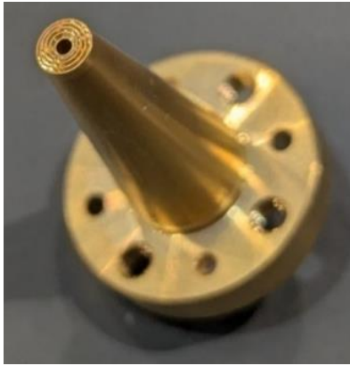
Fig. 2. Final Fabricated WR-03 Feed Horn
