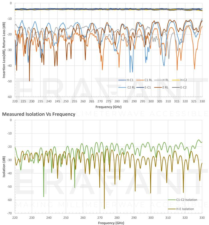
**Measured Insertion Loss and Return Loss Vs Frequency**
