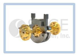
lab or sub-assembly use where frequent connects and disconnects are encountered. In addition, it is also designed for sub-assemblies and lab setup where the waveguide flange connections are in a tight space and not enough room is presented for standard waveguide screw connections. Furthermore, the quick connect provides even pressure on the flanges in order to create a perfect connection that reduces signal leakage due to waveguide misalignment.
