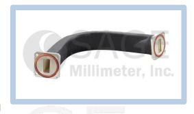
into systems. The flanges of the waveguide are grooved to accept rubber rings to be watertight for outdoor applications. The waveguide is manufactured with a precision manufacturing process to ensure high quality. The waveguide has low insertion loss in the frequency range of 12.4 to 18 GHz. Additional standard lengths and custom length options are available under different model numbers.
