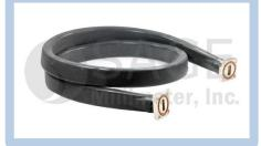
long-term stress free when it is integrated into systems. The flanges of the waveguide are grooved to accept rubber rings to be watertight for outdoor applications. The waveguide is manufactured with a precision manufacturing process to ensure high quality. The waveguide has low insertion loss in the frequency range of 18 to 26.5 GHz. Additional standard lengths and custom length options are available under different model numbers.
