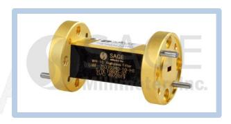
by modifying the design, custom designs can be offered under different model numbers. This particular model features an optimized stepped impedance transformer design and E-plane cut for a smoother transition from the rejection band to the passband.
