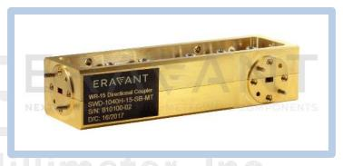
design to achieve a flat coupling level, high directivity, and low insertion loss. The RF ports of the coupler are WR-15 waveguides with UG-385/U flanges. Other standard coupling levels (3, 6, 10, 20, 30, and 40 dB) are available under different model numbers as **SWD-XX40H-15-SB-MT**, where **XX** is the desired coupling level.
