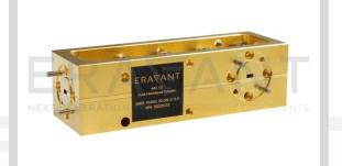
coupler is WR-15 waveguides with UG-387/U-M anti-cocking flanges. Other coupling levels including custom coupling levels and asymmetrical forward/reverse coupling levels are available under different model numbers.
