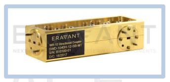
split block design to achieve a flat coupling level, high directivity, and low insertion loss. The RF ports of the coupler are WR-12 waveguides with UG-387/U flanges. Other standard coupling levels (3, 6, 10, 20, 30, and 40 dB) are available under different model numbers as **SWD-XX40H-12-SB-MT**, where **XX** is the desired coupling level.
