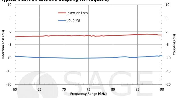
\*Insertion loss includes circuit loss
