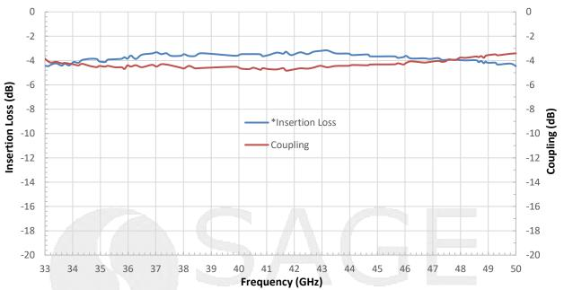
\*Insertion loss includes circuit loss
