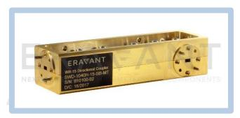
design to achieve a flat coupling level, high directivity, and low insertion loss. The RF ports of the coupler are WR-15 waveguides with UG-385/U flanges. Other standard coupling levels (3, 6, 10, 20, 30, and 40 dB) are available under different model numbers as **SWD-XX40H-15-SB-MT**, where **XX** is the desired coupling level.
