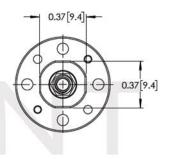
WR-10 WAVEGUIDE W/ UG-387/U-M ANTI-COCKING FLANGE
