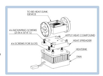
Remount the sub-assembly onto the heatsink main body. Apply heat compound material if desired.
