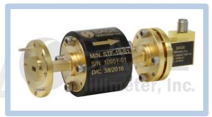
extremely flat output characteristics. The detector is designed to have a 10 MHz video bandwidth and a 1 M $\Omega$  video output impedance. The minimum detectable signal level is approximately -50 dBm. The Faraday isolator is integrated to improve the input port return loss.
