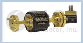
output characteristics. The detector is designed to have a 10 MHz video bandwidth and a 1 M $\Omega$  video output impedance. The minimum detectable signal level is approximately -50 dBm. The Faraday isolator is integrated to improve the input port return loss.
