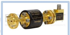
sensitivity and extremely flat output characteristics. The detector is designed to have a 10 MHz video bandwidth and a 1 M $\Omega$  video output impedance. The minimum detectable signal level is approximately - 50 dBm. The Faraday isolator is integrated to improve the input port return loss.
