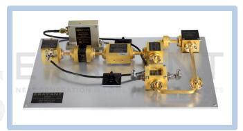
mA. The sensor module is configured with a varactor tuned oscillator, an isolator, an amplifier, a power divider, a circulator and a I-Q mixer. The power divider is used to sample the LO power to pump the mixer, and the circulator is used as a TX/RX diplexer. The varactor has tuning voltage range of 2.8  $V_{DC}$  to +30  $V_{DC}$  and provides ±2.5 GHz tuning bandwidth. Various antennas can be integrated with the module to form sensor heads for many system applications.
