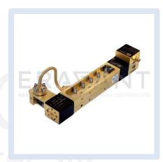
The sensor module is configured with a bias tuned oscillator, an isolator, a directional coupler, a circulator, and a balanced mixer. The directional coupler is used to sample the LO power to pump the mixer, and the circulator is used as a TX/RX diplexer. Various antennas can be integrated with the module to form sensor heads for many system applications.
