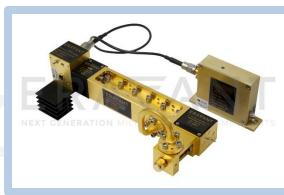
mixer. The sensor module is configured with a mechanically tuned oscillator, an isolator, a directional coupler, a circulator, and an externally biased balanced mixer. The directional coupler is used to sample the LO power to pump the mixer, and the circulator is used as a TX/RX diplexer. Various antennas can be integrated with the module to form sensor heads for many system applications.
