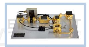
sensor module is configured with a varactor tuned oscillator, an isolator, an amplifier, a power divider, a circulator and a I-Q mixer. The power divider is used to sample the LO power to pump the mixer, and the circulator is used as a TX/RX diplexer. The varactor has tuning voltage range of 2.8  $V_{DC}$  to +30  $V_{DC}$  and provides  $\pm 2.5$  GHz tuning bandwidth. Various antennas can be integrated with the module to form sensor heads for many system applications.
