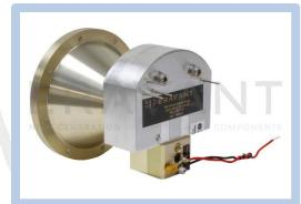
a tuning voltage of 0 to +20 Volts. The sensor heads are configured with a lens corrected antenna, a T/R diplexer, a low noise RF amplifier, an I/Q receiver, an IF amplifier, and a TX/RX oscillator in an integrated package. Sensor heads with a single receiver are offered under model number **SSD-35310-22L-S2** and can only detect the range and speed of a target.
