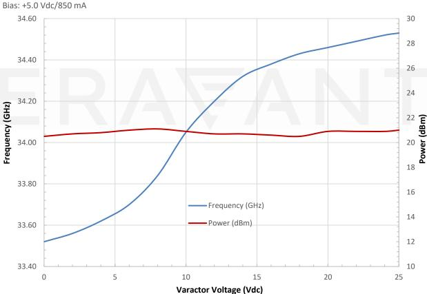
**Typical Frequency and Power Output vs. Varactor Voltage**
