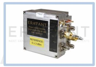
reference is absent. The oscillator delivers a typical output power of +18 dBm and has a nominal harmonic and spurious levels of -25 dBc and -75 dBc, respectively. The oscillator has a built-in voltage regulator to further improve the signal quality and prevent possible damage due to the over voltage operation. The oscillator is hermetically sealed to offer the maximum environmental performance.
