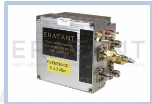
reference is absent. The oscillator delivers a typical output power of +13 dBm and has a nominal harmonic and spurious levels of -25 dBc and -75 dBc, respectively. The oscillator has a built-in voltage regulator to further improve the signal quality and prevent possible damage due to the over voltage operation. The oscillator is hermetically sealed to offer the maximum environmental performance.
