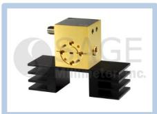
source. The Gunn oscillator's frequency can also be tuned by varying the bias voltage, which is useful for phase-locking and electrical-tuning applications. The Gunn oscillator is equipped with a self-locking set screw for frequency trimming. Models with a micrometer for lab and test bench applications are available under a different model number. The performance of the oscillator can be further enhanced by adding an optional isolator, Gunn oscillator modulator/regulator and temperature heater.
