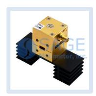
and electrical-tuning applications. The Gunn oscillator is equipped with a self-locking set screw for frequency trimming. Models with a micrometer for lab and test bench applications are available under a different model number. The performance of the oscillator can be further enhanced by adding an optional isolator, Gunn oscillator modulator/regulator and temperature heater.
