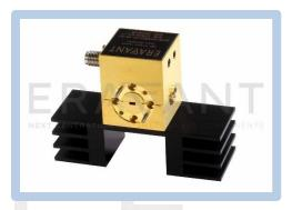
for volume production. The oscillator also delivers low AM/FM noise and harmonic emissions in the wide mechanical and bias tuning range. Compared to its counterparts, such as multiplier-based sources, the Gunn oscillator is an alternative lower cost and cleaner source. The center frequency of the oscillator can be mechanically trimmed via a self-locking set screw within ±1.0 GHz frequency range.
