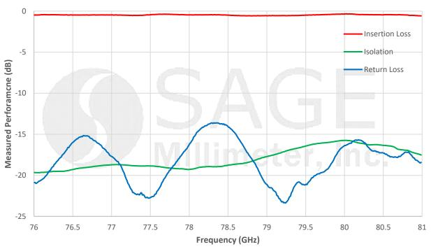
**Note:** The insertion loss, isolation and return loss between other ports, such as port 2 to port 3, port 3 to port 1 are similar to above given plots.
