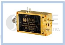
input port configuration is a female K connector and the output is a WR-12 waveguide with a UG-387/U anti-cocking flange. Other port configurations are available under different model numbers.
