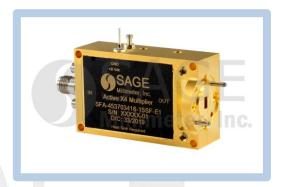
port configuration is a female SMA connector and the output is a WR-12 waveguide with a UG-387/U anti-cocking flange. Other port configurations are available under different model numbers.
