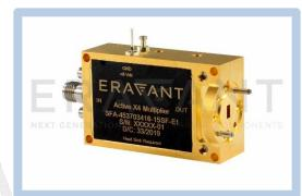
input port configuration is a female K connector and the output is a WR-12 waveguide with a UG-387/U anti-cocking flange. Other port configurations are available under different model numbers.
