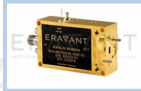
configuration is a female 2.92 mm connector and the output is a WR-12 waveguide with a UG-387/U anti-cocking flange. Other port configurations are available under different model numbers.
