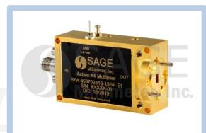
female SMA connector and the output is a WR-15 waveguide with a UG-385/U anti-cocking flange. Other port configurations are available under different model numbers.
