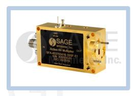
SMA (F) connector and the output is a WR-15 waveguide with a UG-385/U anti-cocking flange. Other port configurations are available under different models. This model is tested to operate in the extended temperature range of  $-40^{\circ}$  C to  $+85^{\circ}$  C.
