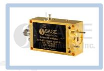
for the multiplier is +8 V<sub>DC</sub>/400 mA. The input port configuration is a K(F) connector and the output is a WR-15 waveguide with a UG-385/U anti-cocking flange. Other port configurations are available under different models.
