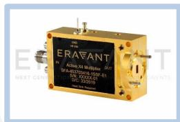
port configuration is an K (F) connector and the output is a WR-15 waveguide with a UG-385/U anticocking flange. Other port configurations are available under different models.
