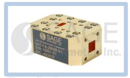
forms. The OMT shows high port isolation while providing a low insertion loss. The OMT is configured with a  $0.280^{\circ}$  x  $0.280^{\circ}$  square waveguide for the antenna port and two WR-28 waveguides for the horizontal and vertical ports. All ports have standard UG-599/U flanges and 4-40 threaded holes.
