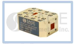
forms. The OMT shows high port isolation while providing a low insertion loss. The OMT is configured with a  $0.280'' \times 0.280''$  square waveguide for the antenna port and two WR-28 waveguides for the horizontal and vertical ports. All ports have standard UG-599/U flanges and 4-40 threaded holes.
