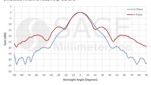
WR-90 Rectangular Horn Antenna, 20 dBi Gain with N Type Coax Connector
