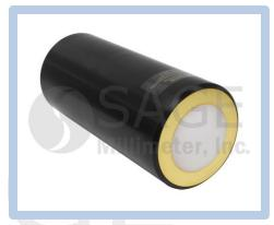
efficiency and low side lobe levels are achieved with a low loss lens. A weather resistant configuration makes the antenna suitable for outdoor use. The horizontal and vertical ports are WR-28 waveguides with UG-599/U flanges and 4-40 threaded holes.
